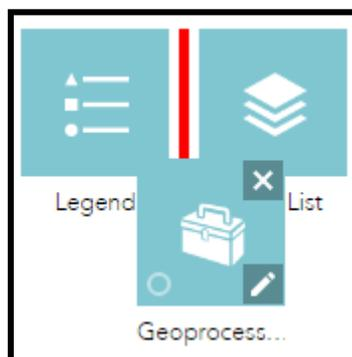
5. You can also group in-panel widgets by dragging one or more widgets into another widget. The grouped widget shows as a folder icon on the controller widget. To ungroup the widget, drag each widget out of the group.
