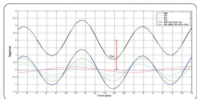
Figure 5: Harmonic Waves that Forms Tidal Height, Hery Purwanto (2005)
