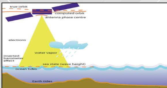
Figure 2.2: Corrections for Altimeter Range Measurements (Bosch, 2010)
