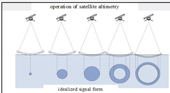
Figure 2.1: Footprint development (Courtesy of W. Bosch - Satellite Altimetry, ESPACE, 2010)
