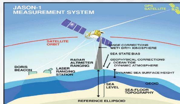
Figure 2.3: Principle of Satellite Altimeter (Courtesy of AVISO)
