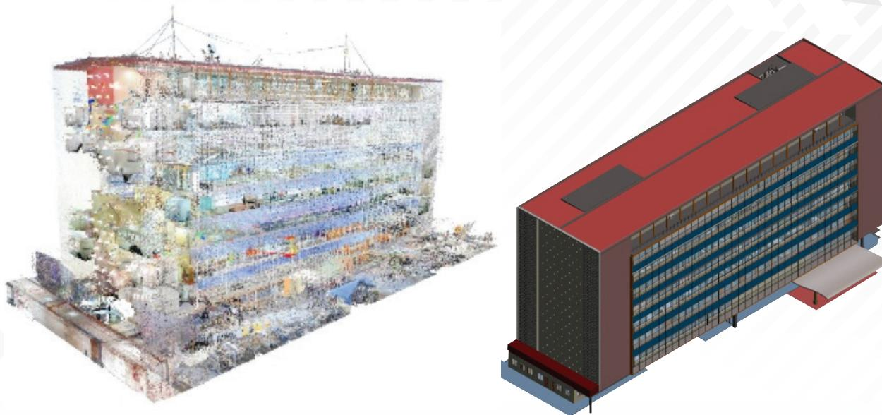
Figure 2: DSMM Bangunan Ukur in Point Clouds (left) and in BIM Model (right)
